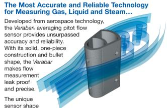
reduces drag and flow induced vibration. The location of the low-pressure ports eliminates the potential for clogging and improves signal stability.
