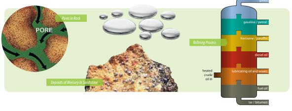
Where these contaminants end up in the plant depends on many factors. Mercury as suspended vapour in the product will act in the same way as many other oil and gas products. During fractional distillation temperature and pressure changes allow vapours to condense into selected by-products.
