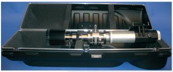
due to superior fused glass design. Superior lighting allows crude oil to become easy to monitor. CANTYVISIONCLIENT™ software is installed on a user-supplied PC, and connected to the InFLow™ measurement system via Gigabit Ethernet network. Live images of the process can be viewed from any networked PC. The live images are remotely analyzed by CantyVisionClient  $^{\text{TM}}$  software.
