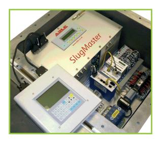
The ABLE SlugMaster® uses two ultrasonic flowmetering technologies and a smart PLC to intelligently choose which technology to use, based on the process conditions. Constant metering is achieved regardless of solids and gas contamination. The change over between the two metering technologies is calculated with unique mathematical software, which enables exceptional measurement accuracy.
