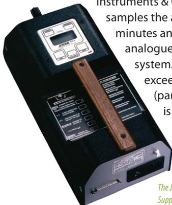
*The Jerome 631-XE Hydrogen Sulphide Analyser
