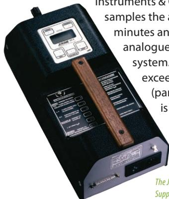
*The Jerome 631-XE Hydrogen Sulphide Analyser
