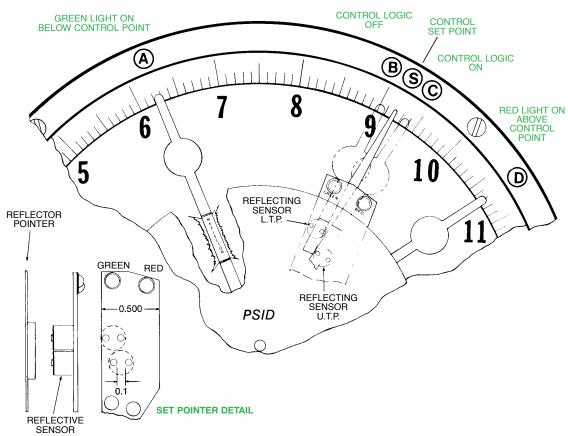
FIGURE 1 — Locked Logic control arrangement
