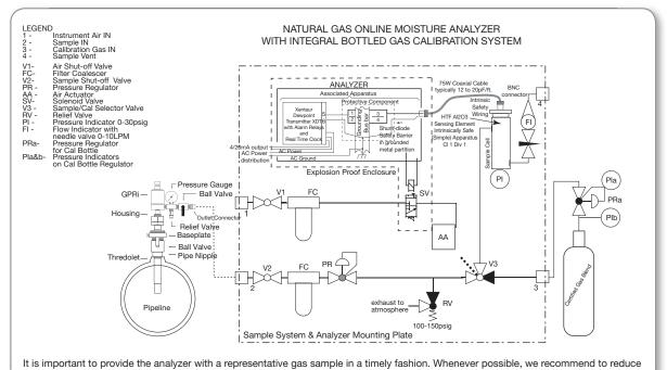
sample pressure at the pipeline. This will reduce the risk for condensation in the sample lines and shorten sample transport to the analyze Shown here is an insertion probe regulator with integrated membrane filter that reduces the pressure without requiring heating.
