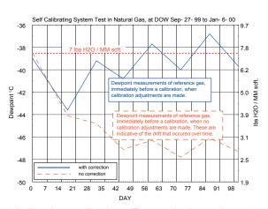
challenging applications. The graph above shows 90 days of dewpoint monitoring data with calibration adjustment in an applications where glycol carryovers have prevented conventional systems from performing. After a settling period of two weeks, the system has reliably provided accurate results.
