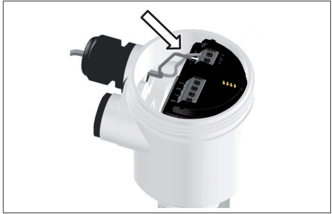
Fig. 27: Connection steps 5 and 6 - Single chamber housing
