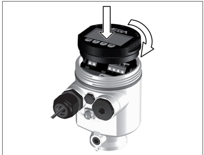
Fig. 33: Insertion of the indicating and adjustment module with single chamber housing into the electronics compartment
