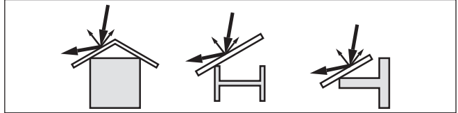
Fig. 18: Cover smooth profiles with deflectors
