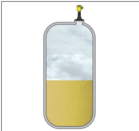
Fig. 6: Level measurement in an acid tank with VEGAPULS 61
