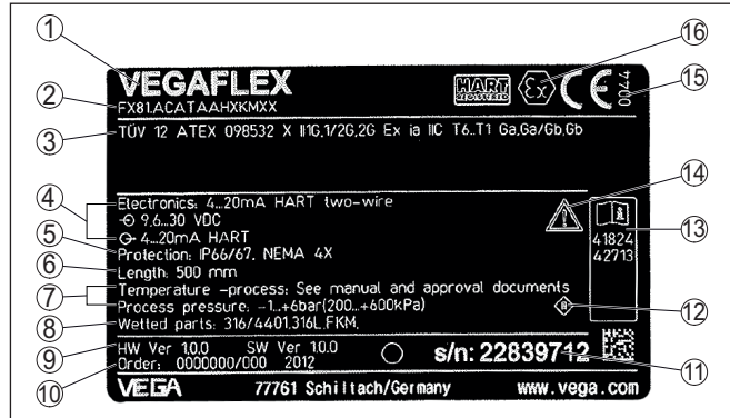
Fig. 4: Layout of the type label (example)
