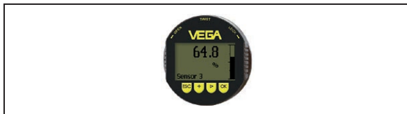
Fig. 24: Display and adjustment module PLICSCOM
