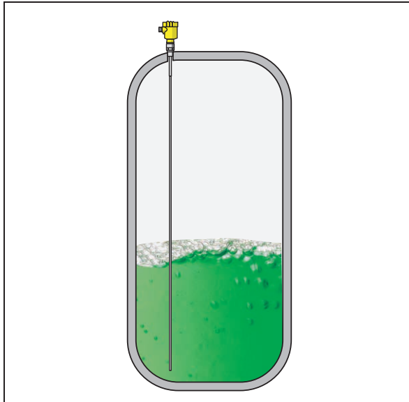
Fig. 15: Level measurement in a storage vessel with VEGAFLEX 81
