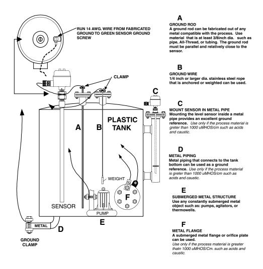
Figure 2-5 Customer-Fabricated Ground References
