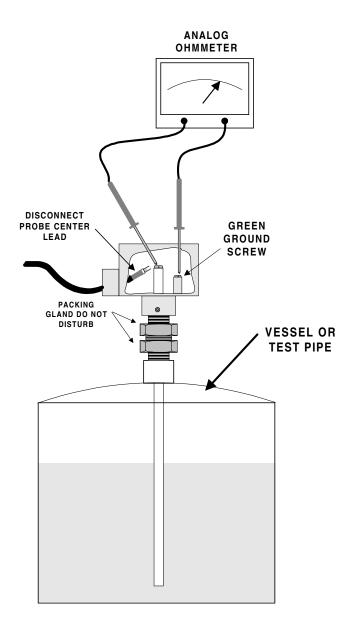
Figure 4-5 Checking the Sensing Element
