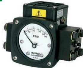
**Model 140 & 142 “Delta Meters”** are available with either one or two hermetically sealed reed switches for either high alarm, low alarm, or both and a 4-20mA transmitter depending on model. The switches are Single Pole Double Throw (SPDT) or Single Pole Single Throw (SPST) with adjustable set points. Switches can be set to activate/deactivate on rising or falling pressure.
