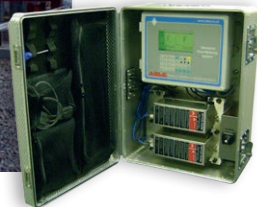
Self-powered flow computer incorporated in Aluminium case
