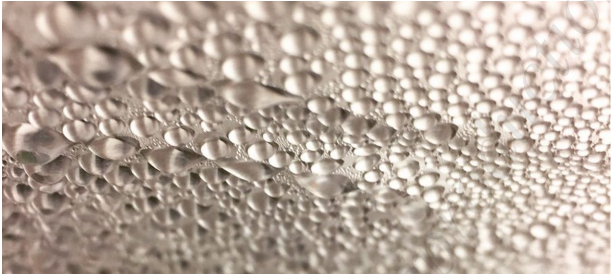
Fig.3 Image of condensates on pipe wall inner surface
