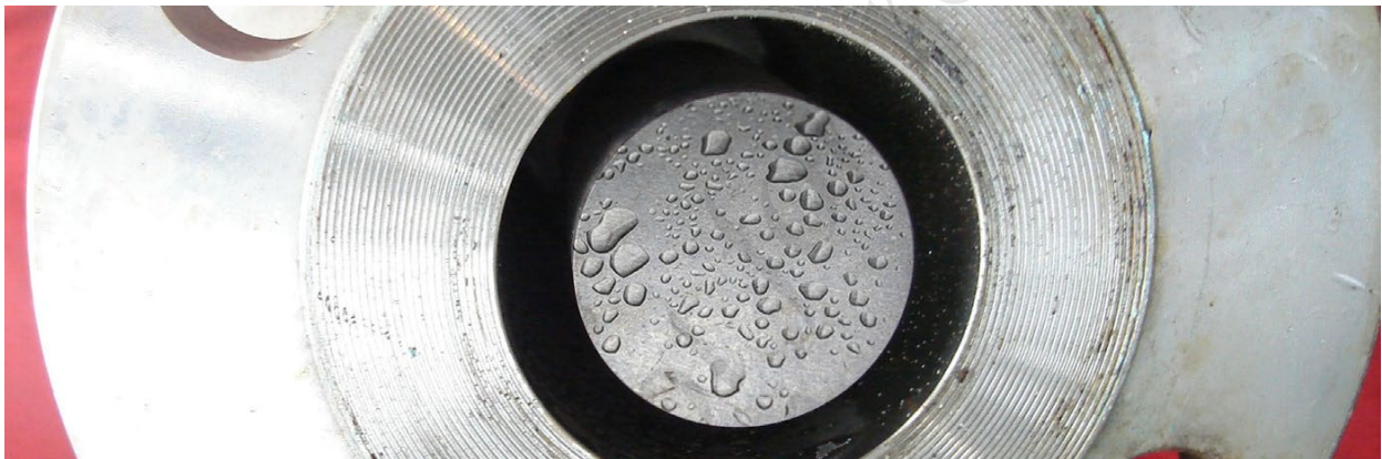
Fig.4 Image of condensation on ultrasonic transducer probe face
