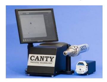
In September 2019, the S·O·S<sup>sm</sup> Services regional laboratory in Peoria evaluated the Canty Fuel / Lube Oil Particle and Water Analyser for its suitability as a particle counting solution in the S-O-S Services programme. The instrument provided ISO 4406 particle count results with similar repeatability to other particle counting instruments in the marketplace. This instrument was deemed an acceptable device for particle count analysis in the S-O-S Services programme.
