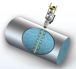
The FPI Mag operates based on Faraday's Law of Electromagnetic Induction: When water (a conductor) moves through a magnetic field, it produces a voltage that is directly proportional to the velocity of the conductor.
