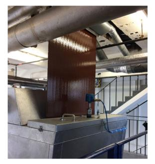
For the production of Denso Tape, mixing tanks are filled with the petrolatum, which is maintained at a temperature of approximately 165°C to avoid solidification, and applied to the synthetic fabric before being fed by rollers through a water quenching tank to the final cutting process.
