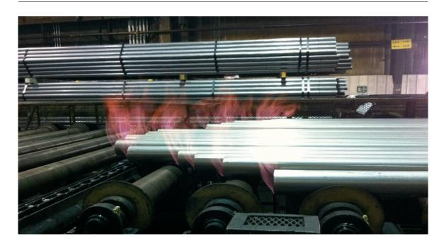
Heat treatment processes for metals represent harsh environments for the measurement of blanket gas constituents. Ambient conditions in the furnaces have high particulate levels, acid gases and other compounds either outgassing or being burned off of the metal components being processed.
