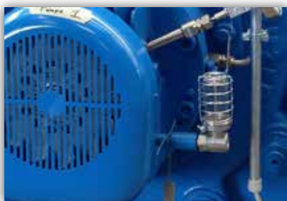
Watchdog Oiler mounted on centerline of desired oil level
