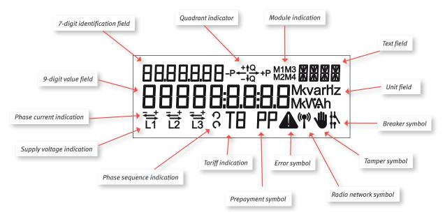
9-digit value field: This field is used for displaying register values.
