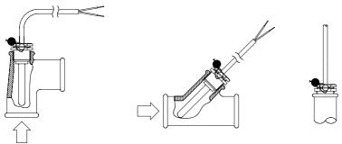
The temperature sensors should reach the bottom of the pockets. If a short response time is required, "non-hardening" heat conducting paste can be used.
