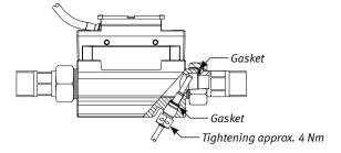
The flow meter can be used in both PN16 and PN25 and can be supplied marked either PN16 or PN25 as desired.
