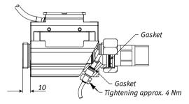
Straight inlet: MULTICAL® 402 requires neither straight inlet nor straight outlet to meet the Measuring Instruments Directive (MID) 2004/22/EC and EN 1434:2007. A straight inlet section will only be necessary in case of heavy flow disturbances before the meter. We recommend to follow the guidelines of CEN CR 13582.
