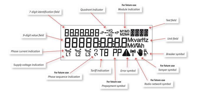
9-digit value field: This field is used for displaying register values.
