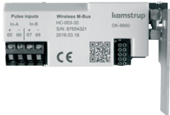
\* The wireless M-Bus module must be connected to an internal or external antenna. When mounting an external antenna ensure that the antenna cable is not jammed or damaged when the calculator is assembled. Before mounting or replacing modules the power supply to the meter must be switched off. The same applies to mounting of an antenna.
