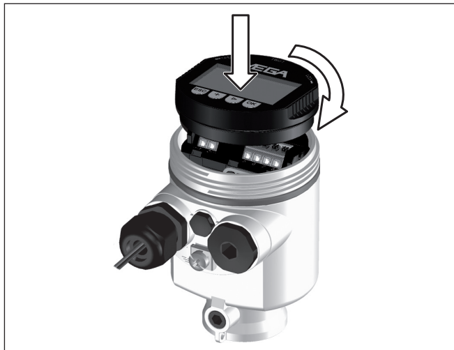
Fig. 22: Insertion of the indicating and adjustment module with single chamber housing into the electronics compartment
